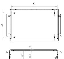
AVAILABLE SPACE INSIDE THE PENDANT CONTROL PANEL WITH AND WITHOUT THE WIRING PLATE
